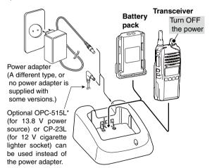
\*CAUTION: NEVER connect the OPC-515L to a power source using reverse polarity. This will ruin the battery charger White line:
