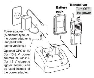
\*CAUTION: NEVER connect the OPC-515L to a power source using reverse polarity. This will ruin the battery charger White line: (+) Black line: (-)
