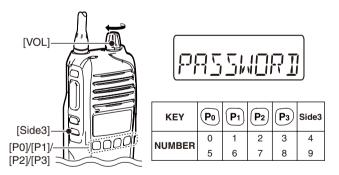
③ When the "PASSWORD" indication does not clear after inputting 4 digits, the input code number may be incorrect. Turn OFF the transceiver and start over in this case.
