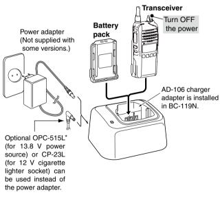
\*CAUTION: NEVER connect the OPC-515L to a power source using reverse polarity. This will ruin the battery charger.
