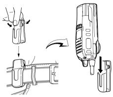
(5) Once the transceiver is locked in place, it swivels as illustrated below.
